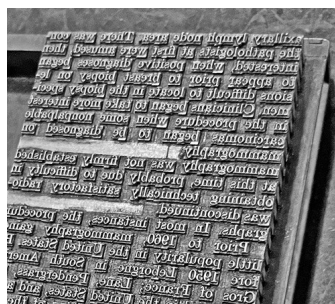
A working 1936 Linotype (above left) is demonstrated at the Baltimore Museum of Industry. Invented by German immigrant Ottmar Mergenthaler (top right), the machine creates lines of metal type (above right) ready for printing on a press.
