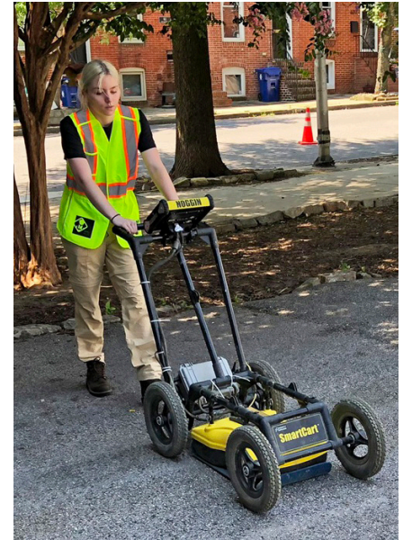
Above left: Old sand mines were discovered beneath the 600 block of E. Clement Street in the summer of 1951. This photo from The Baltimore Evening Sun (July 7, 1951) shows workers at the bottom of one of the 30-foot shafts dug through the street. Above right: Technician conducts a ground-penetrating radar survey on the block in June 2024. Photo by Steve Cole.
