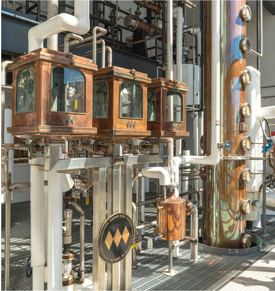
Left: Sagamore Spirit distillery uses a triple-distillation process where the alcohol is repeatedly converted from liquid to vapor and back again. At each step, the liquid can be observed in a series of three “spirit safes.” Photos by Mary Braman.
