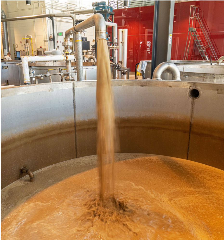
“Sour mash” is piped into a 6,500-gallon “bubbling tank” at the distillery. With yeast added, the mixture ferments for three days before the distillation process begins. Photo by Mary Braman.
